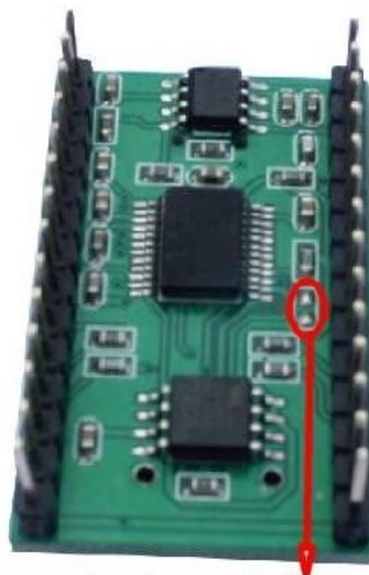
Unpopulated space for on-board Mode Selection on the 28P
